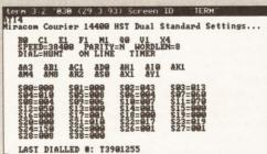
The command ATIn - in this case, ATI4 - is the enquiry command. Here's the reply Wavey got. dial the Compulink Information eXchange number. (Most modems have a limit of 40 characters in the command string, not including the AT prefix, spaces, or carriage returns.)
