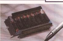
Expand your A500's memory up to a total of 2MB without disposing of you existing 512K upgrade (works with 1MI chip RAM, 512K RAM must be 4 chip type or not exceeding 9cm in length. You Amiga needs to be opened, this may effect your warranty).
